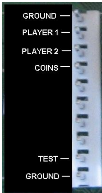
Figure 8. 10 Pin Molex connector pin layout
